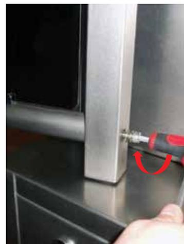
3. Tighten bottom fixing screw
