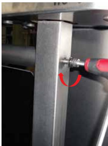
2. Tighten top fixing screw
