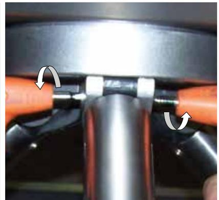
3. Tighten screws with 5 mm. keys
